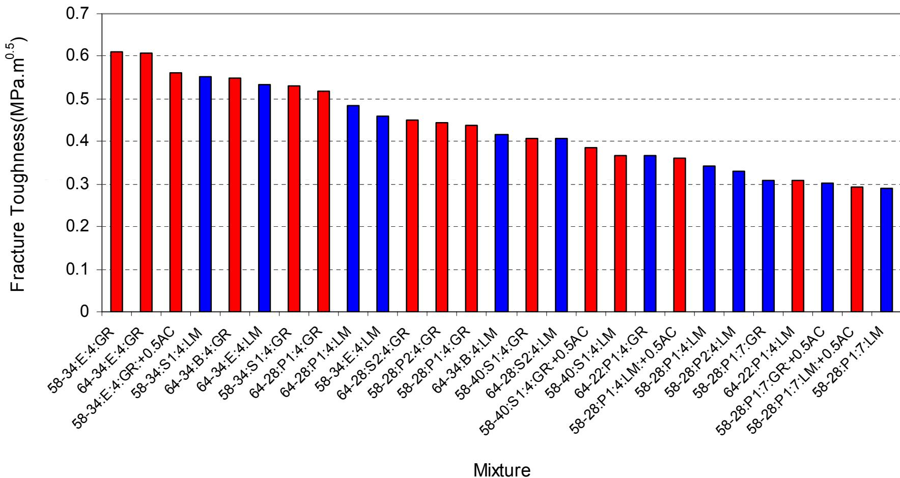
Fracture Toughness Ranking at  $T_H$
