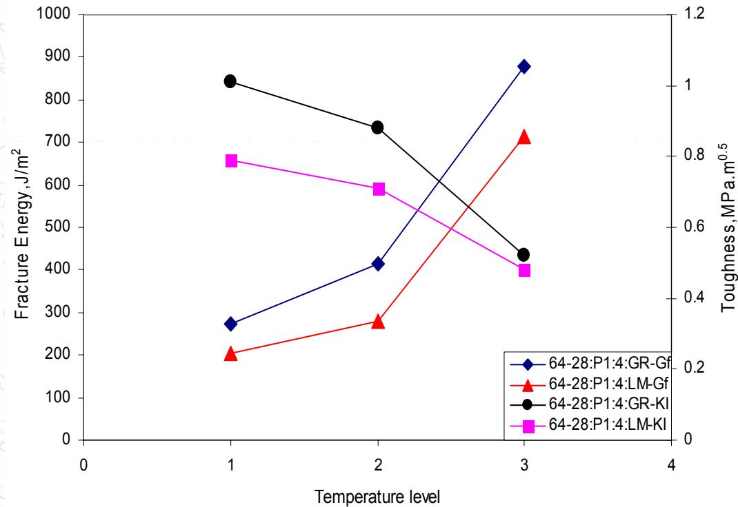
Mean fracture toughness granite > Mean fracture toughness limestone
