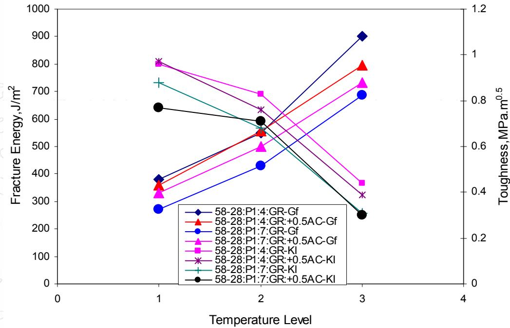
Mixtures with 4% air void overall have higher fracture toughness and fracture energy than mixtures with 7% air void specimens
