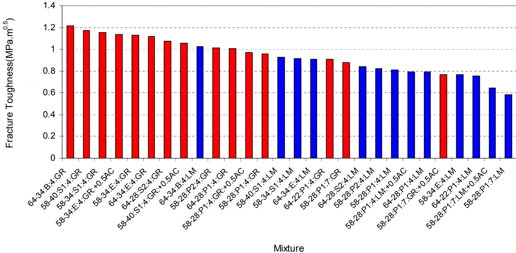
Fracture Toughness Ranking at  $T_L$
