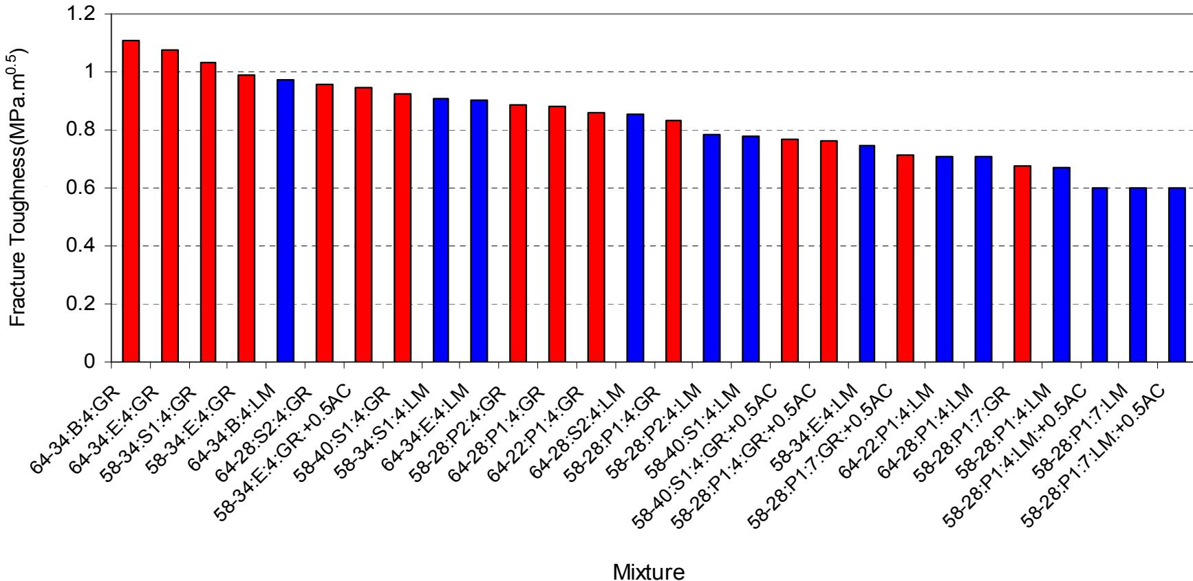
Fracture Toughness Ranking at  $T_M$
